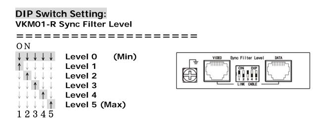
Sync Filter is designed for using UTP CAT5 cabling.
